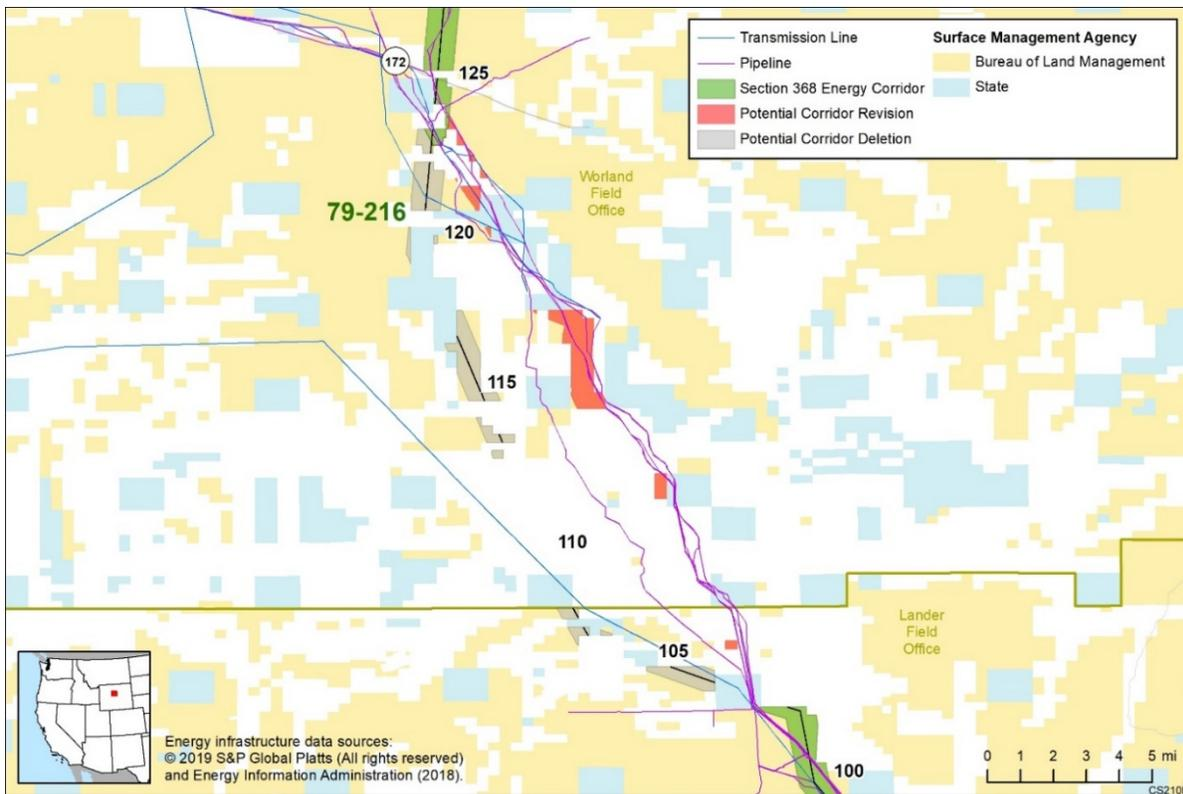
Figure 3.5-39e. Potential Revision to Corridor 79-216 (MP 103 to MP 125)
