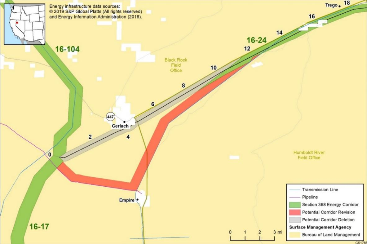
Figure 3.5-15c. Potential Revision to Corridor 16-24 (MP 0 to MP 12)
