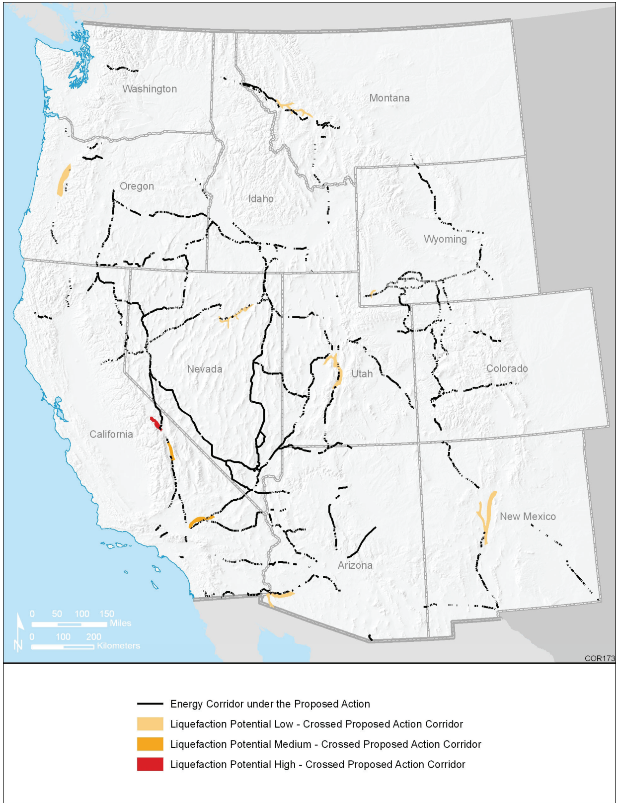
FIGURE 3.14-3 Liquefaction Hazards in the 11 Western States under the Proposed Action
